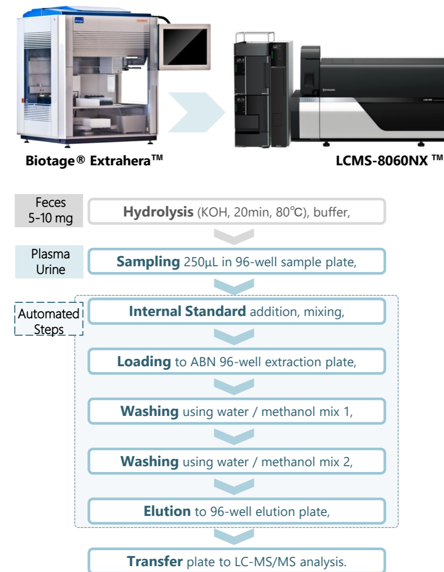
Figure 1. Pretreatment Protocol (Plasma, Urine, Feces). Details of this protocol are provided in the Method Package.
