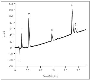
Figure 1: Chromatogram for atenolol (1), pindolol (2), metoprolol (3) propranolol (4) and alprenolol (5) separated on an Accucore C18, 2.6  $\mu$ m, 50 x 2.1 mm column.
