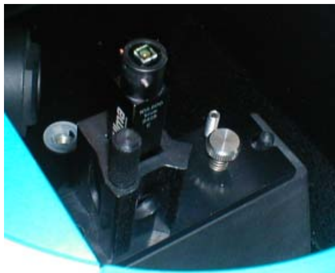
Figure 5 TrayCell with sample mounted for analysis.
