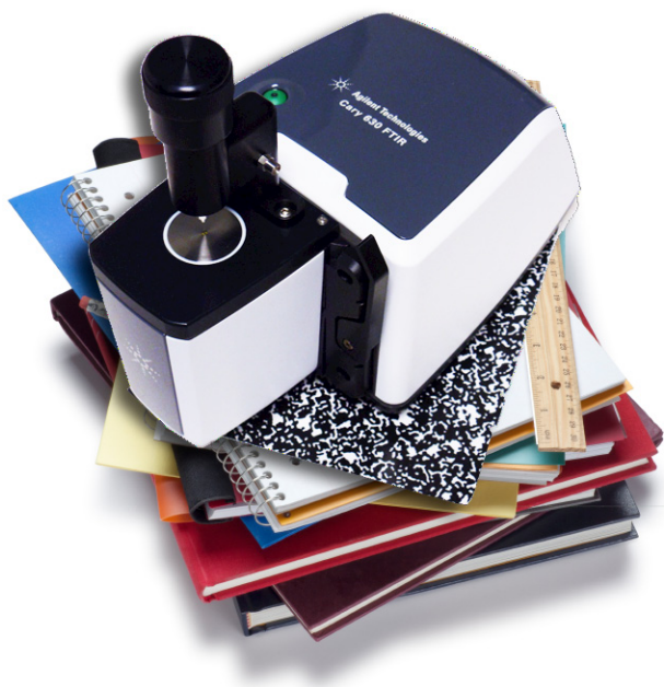
Figure 1. The Agilent Cary 630 FTIR spectrometer (all photographic elements shown in context)
