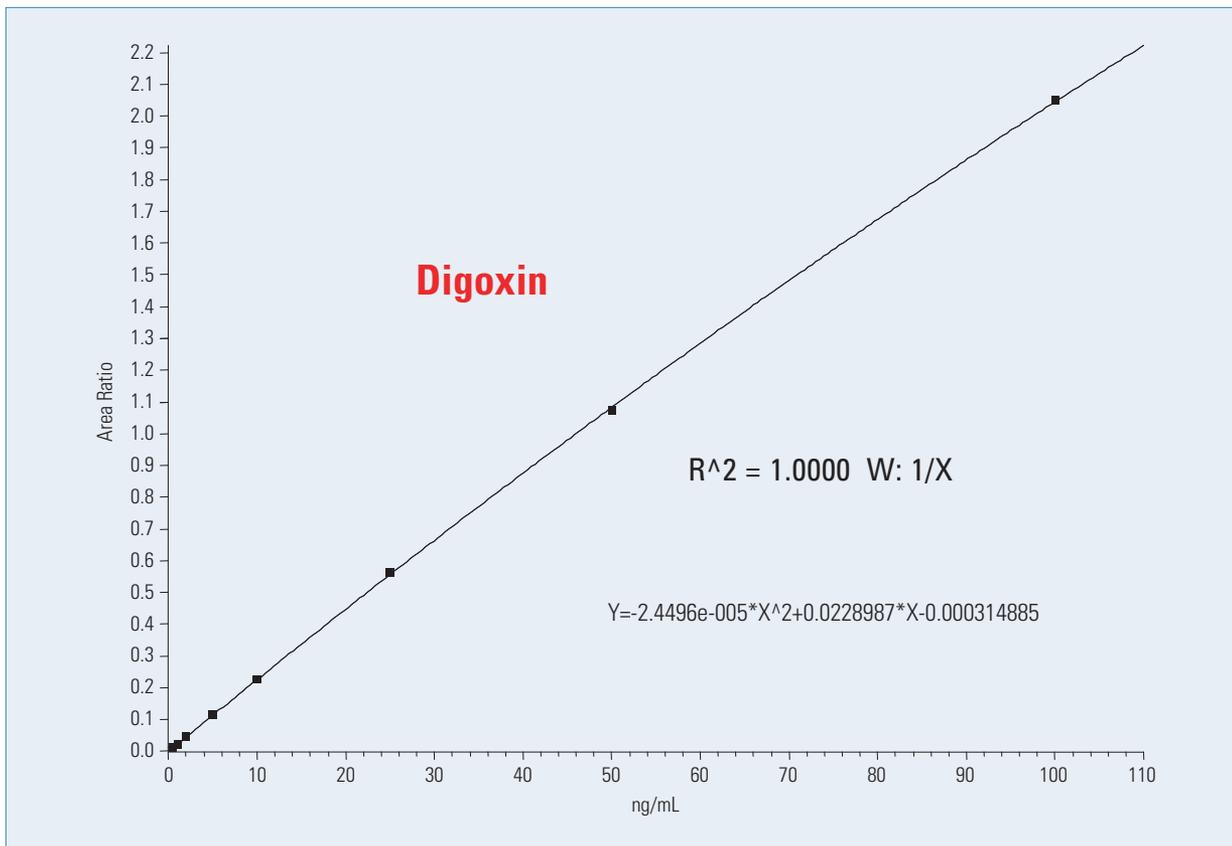
Figure 3: Representative calibration curve from standards spiked in serum
