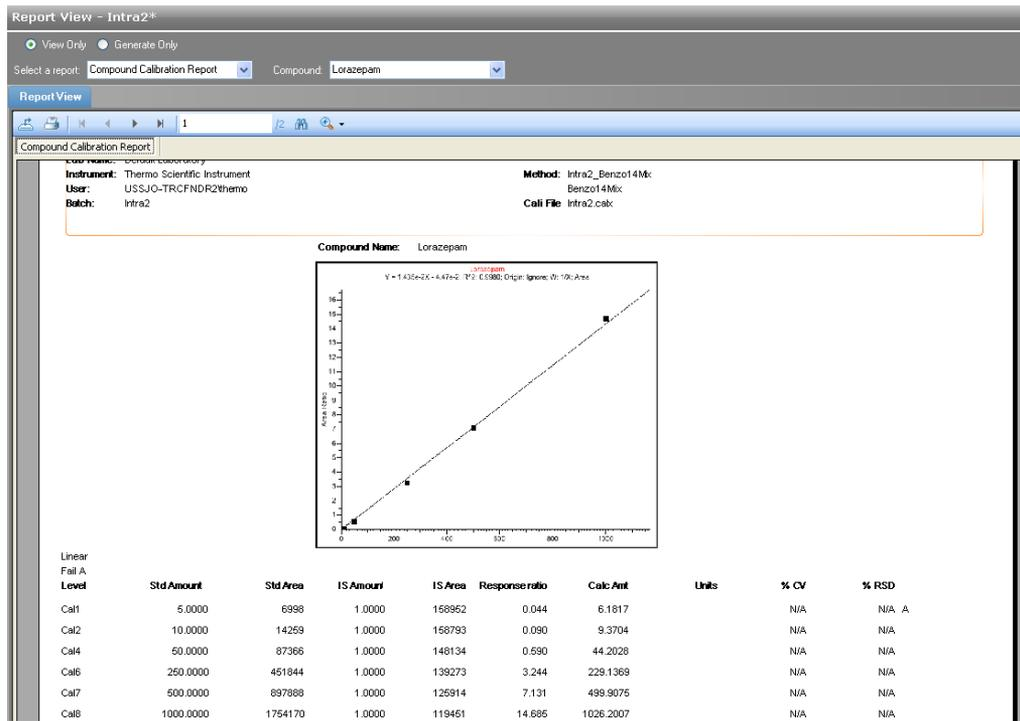
Figure 8. Compound Calibration Report for lorazepam
