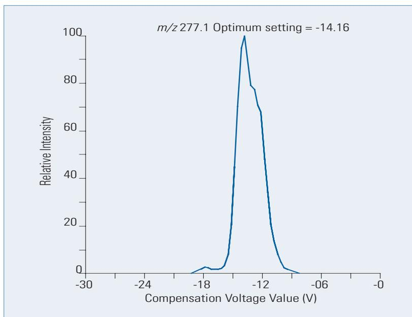
Figure 2: Compensation voltage scan from the infusion of a clenbuterol reference standard. The maximum response for clenbuterol occurred at a compensation voltage of -14V.
