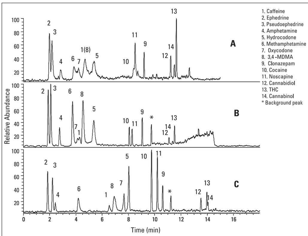
Figure 1: Comparison of 1.9  $\mu\text{m}$  Hypersil GOLD stationary phases for the UHPLC separation of 14 illicit drugs. A) Hypersil GOLD aQ, Method A was applied; B) Hypersil GOLD, Method B was applied; C) Hypersil GOLD PFP, Method C was applied. See Appendix A for methods details.
