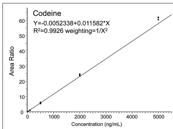
Figure 5. Calibration curve of codeine in human urine
