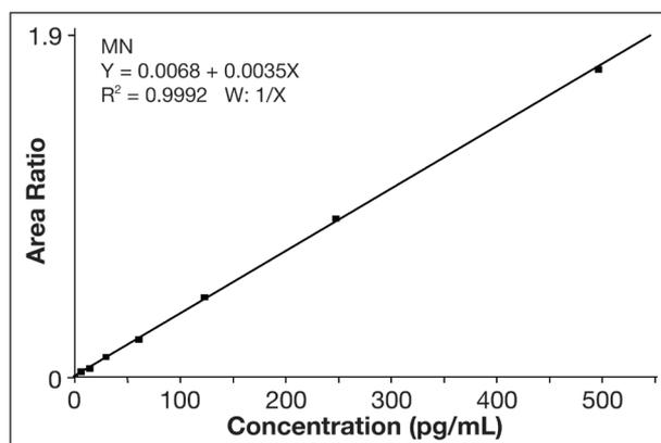
Figure 2. Calibration curve of MN in CSS
