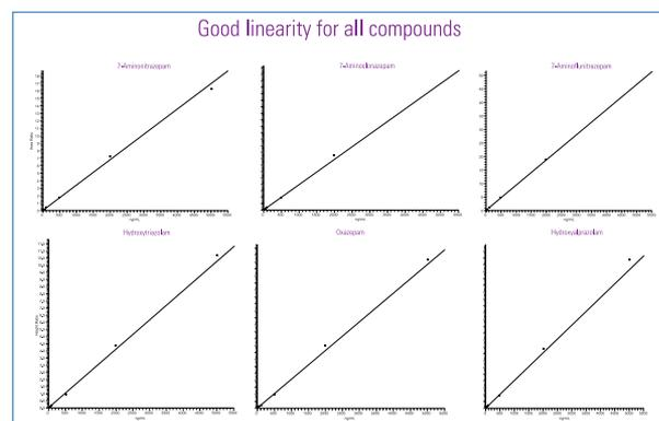
Figure 2: Calibration curves (10-5000 ng/mL) for all analytes
