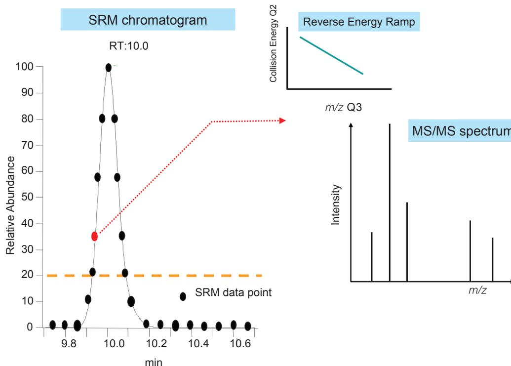
Figure 1: QED detection mode: when a monitored SRM transition reaches a targeted threshold, a full MS<sup>2</sup> spectrum is acquired using a Reverse Energy Ramp scan.
