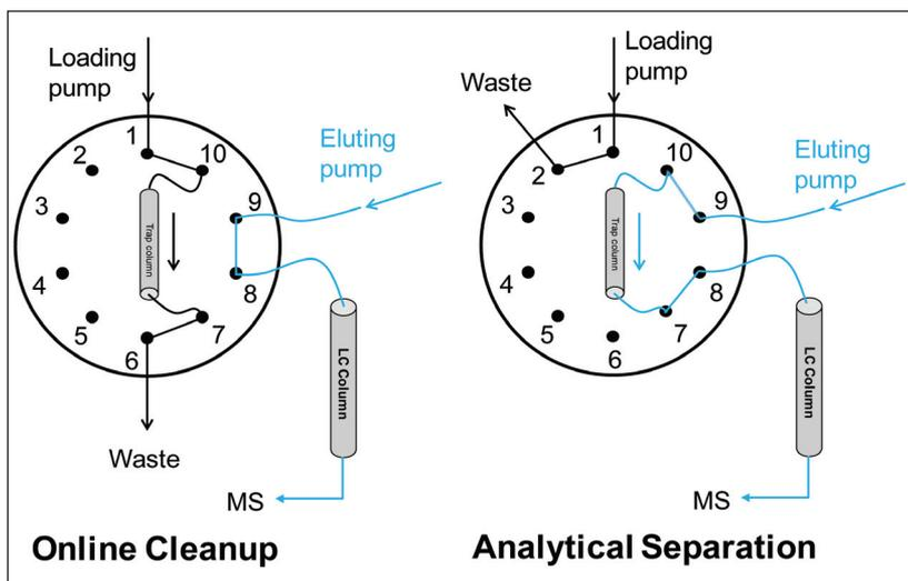
Figure 1. Microflow LC setup with pre-concentration trapping column
