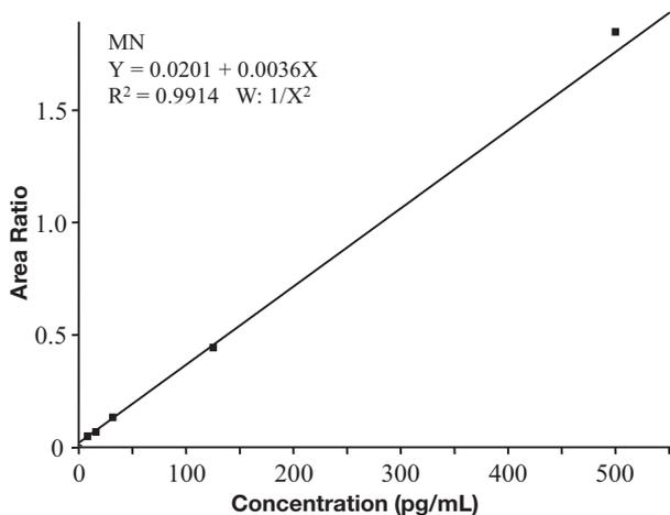
Figure 3. Calibration curve of MN in CSS
