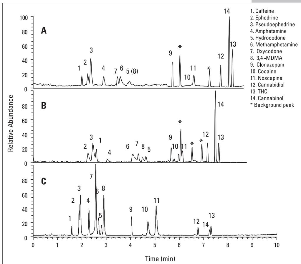
Figure 3: Comparison of hybrid stationary phase chemistry for the separation of 14 illicit drugs. A) 50 x 2.1 mm Hypersil GOLD + 50 x 2.1 mm Hypersil GOLD PFP, Method F; B) 50 x 2.1 mm Hypersil GOLD PFP + 50 x 2.1 mm Hypersil GOLD, Method G; C) 100 x 2.1 mm Hypersil GOLD PFP + 20 x 2.1 mm Hypersil GOLD, Method H. See Appendix A for method details.
