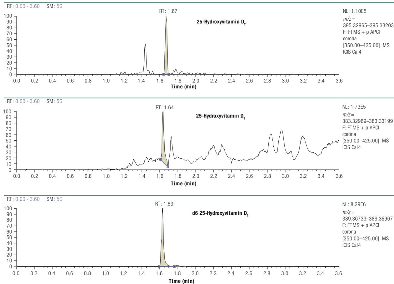
Figure 3. Chromatograms at LLOQ of 2 ng/mL with 50 ng/mL internal standard
