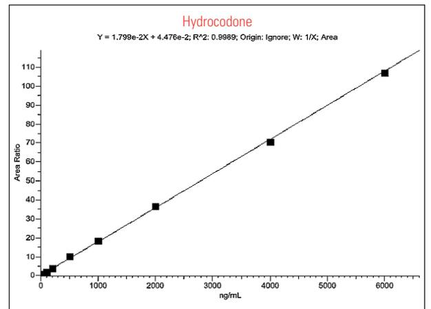
Figure 1. Representative calibration curves for opiates in urine
