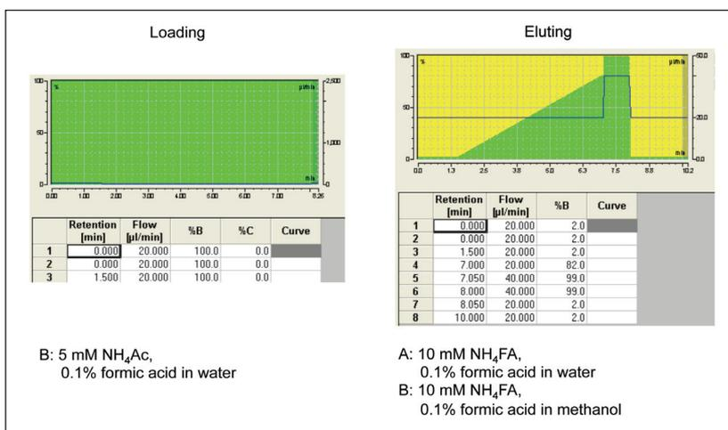
Figure 2. LC gradients of microflow LC with online clean-up
