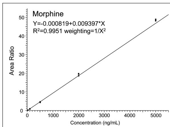
Figure 4. Calibration curve of morphine in human urine
