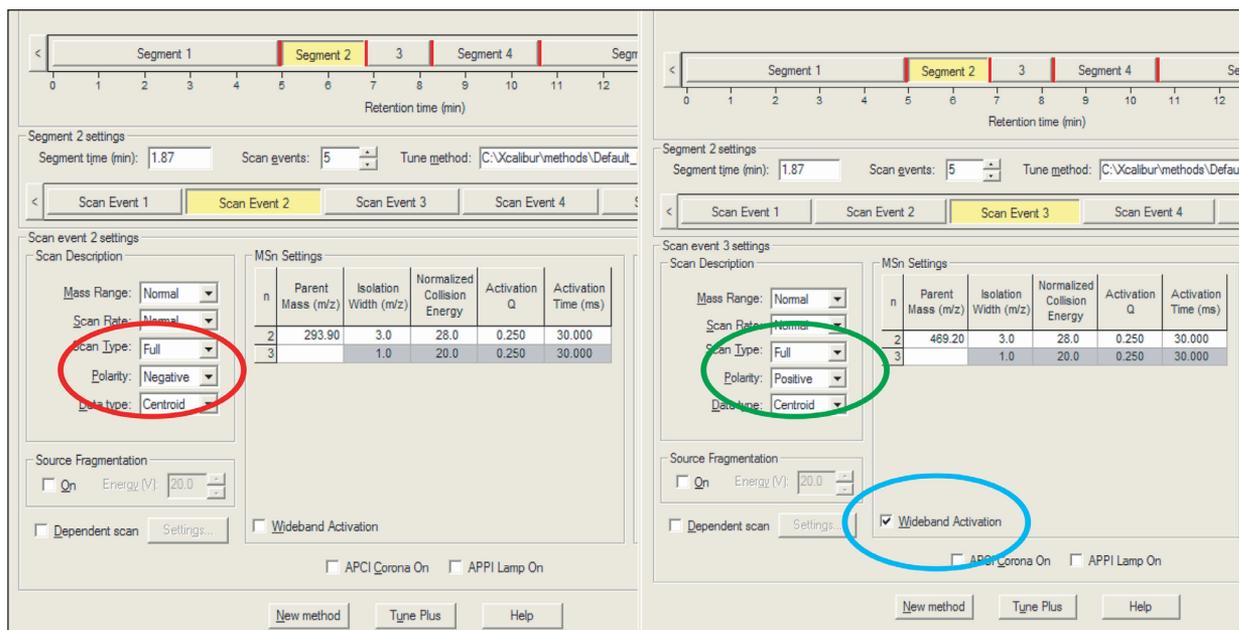
Figure 1: Instrument Setup settings for chlorothiazide (segment 2, scan event 2) and cromolyn-Na (segment 2, scan event 3)
