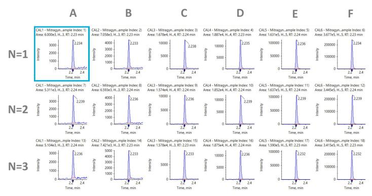
Figure 4: Extracted Ion Chromatograms (XICs) of the Quantifier MRM of Mitragynine (n=3). Replicates are shown across the following range of concentrations (A) 2 ng/mL; (B) 5 ng/mL; (C) 10 ng/mL; (D) 20 ng/mL; (E) 100 ng/mL; (F) 500 ng/mL.
