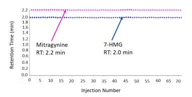
Figure 3: Retention Time Reproducibility of Method. Metric plot of retention time across 70 injections highlights the high chromatographic reproducibility of the method.
