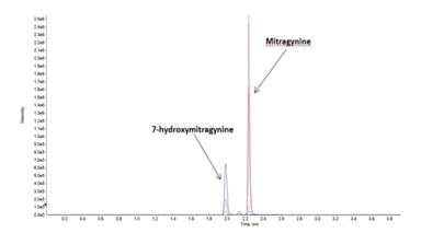
**Figure 2: Chromatogram Showing the Elution Profile of Analytes.** Using targeted MRM detection, mitragynine and 7-HMG were detected at 2.22 and 1.96 min, respectively, when using the optimized LC method.
