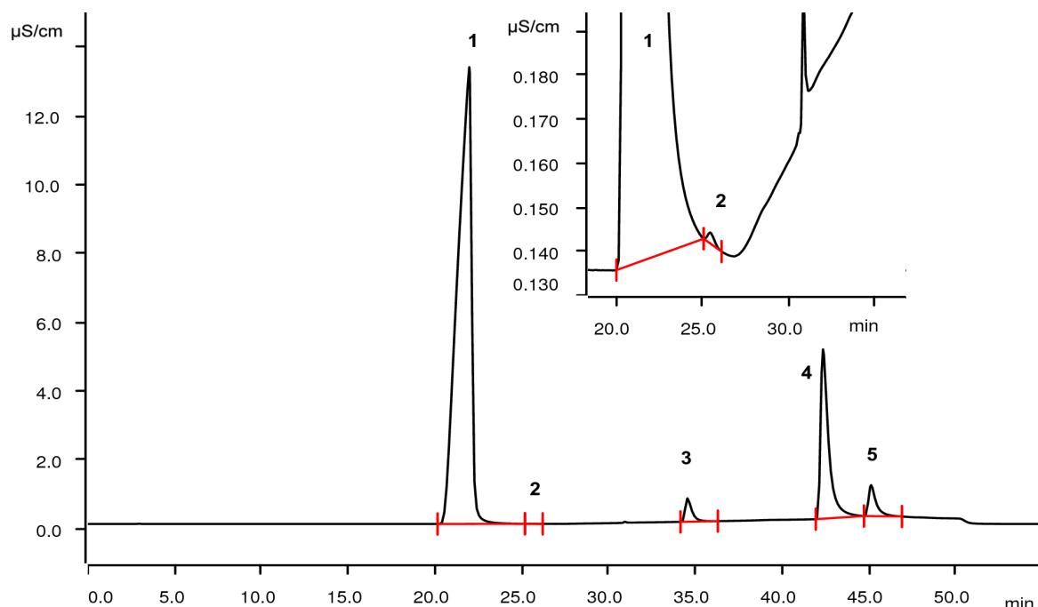
Cation analysis by IC in wastewater is a proven method. Limiting factor is often the Na/NH<sub>4</sub> separation. High sodium concentrations may make ammonium determination impossible due to peak overlapping. The use of sequential suppression and a Dose-in gradient improve the Na/NH<sub>4</sub> separation and enables determination of low ammonium concentrations.
