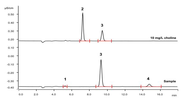
Succinylcholine is a short-term paralyzing agent used e.g., for tracheal intubation. Choline is a building block of the drug and needs to be determined as an impurity. USP applies cation chromatography with conductivity detection after suppression. Eluent composition and column type do not exactly comply with the USP method. However, the results fulfill the respective requirements. The choline concentration of the sample is out of USP specifications.
