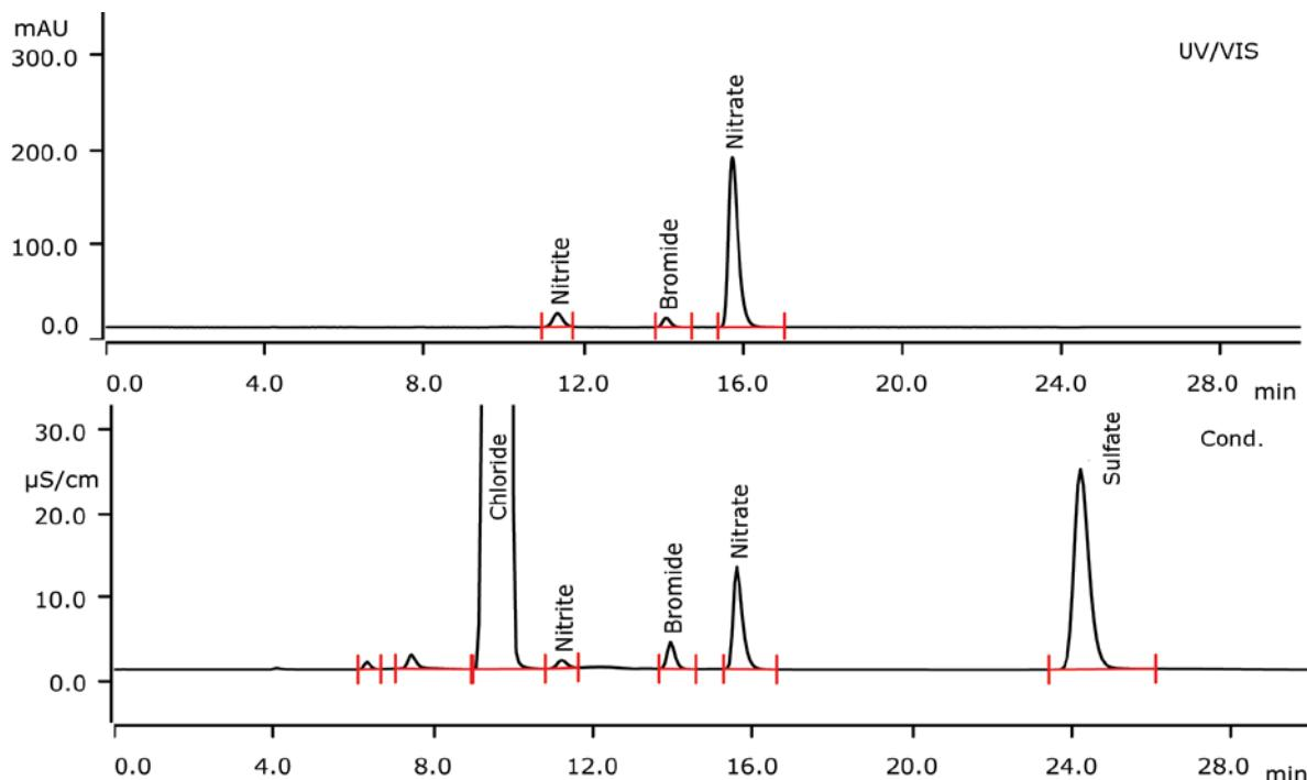
The determination of low nitrite concentrations besides excess sodium chloride is demanding due to the small retention time difference of these two anions. Dual detection – conductivity and UV/VIS – is a powerful means to accurately determine nitrite traces in a 20 g/L chloride matrix. The UV/VIS chromatogram shows no chloride interferences. AN-C-145 shows the determination of ammonium traces besides excess sodium.
