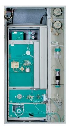
The Process IC is available with either one or two measurement channels, along with integrated liquid handling modules and several automated sample preparation options.
