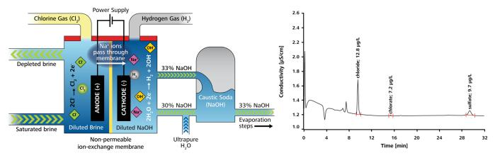
*Left: Diagram of the membrane-cell technique used to produce concentrated NaOH and KOH alongside Cl*<sub>2</sub> (source material: www.eurochlor.org). *Right: 100 μL injection of 50% KOH sample (diluted 1:10), using Metrohm Inline Sample Preparation (MISP) techniques for extra application flexibility.*
