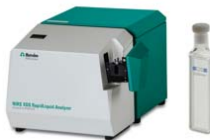
Fig. 1: A NIRS XDS Rapid Liquid Analyzer equipped with a NIRS quartz glass cuvette of 1 mm path length was used to record the spectral data.
