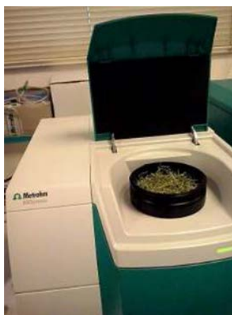
Fig. 1: A NIRS DS2500 analyzer was used to record the representative spectra.
