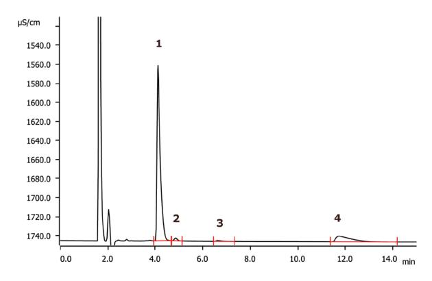
Before the liquefaction process of the natural gas, carbonate and hydrogen sulfide need to be removed through a scrubber solution containing piperazine and N-methyl diethanolamine (MDEA). The concentration ratio of the two components is determined by ion chromatography on a Metrosep C 4 - 150/4.0 column applying direct conductivity detection.
