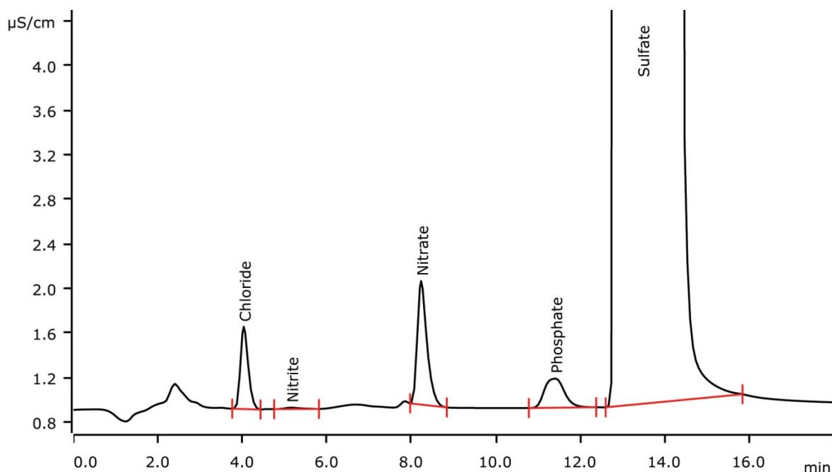
Determination of chloride and sulfate (not quantified) in a highly viscous petrochemical sample applying sample combustion followed by anion chromatography with conductivity detection after sequential suppression. The sample has a particularly high sulfate content.
