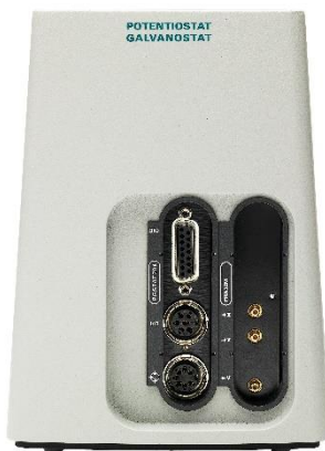
Figure 2 – The Metrohm Autolab PGSTAT204, equipped with the FRA32M module.
