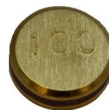
Figure 3 - Standard resistor used in this study. The number 100 refers to the approximate resistance of 100 \Omega .
