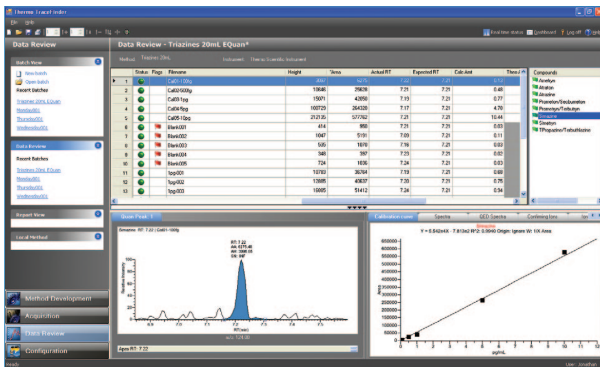
Figure 5. Data Review section. The red flags for blank samples indicate that peaks were not found in these samples.
