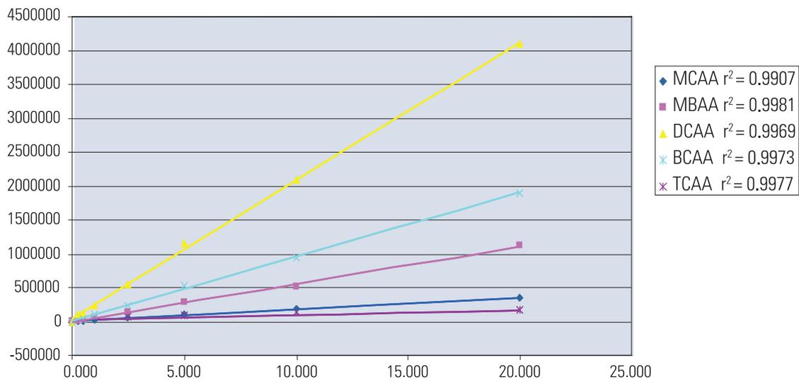
Figure 4: Calibration curve overlay of the HAA compounds in water by IC-MS/MS
