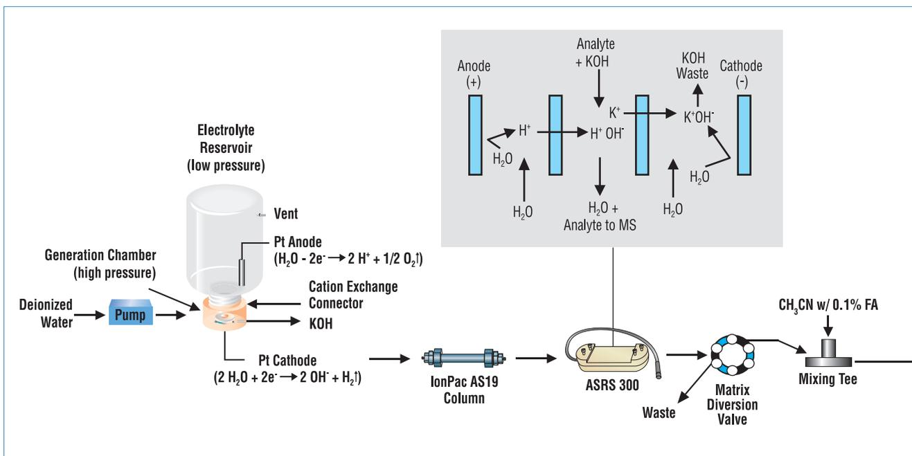
Figure 1: Flow schematic of the IC-MS/MS system
