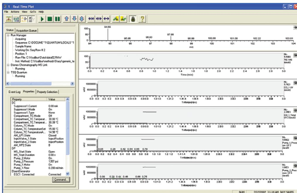
Figure 2: These chromatograms show the progress of the pump pressure and front end detector data along with the TSQ Quantum Access MS data. The left side of the screen shows the status of the ion chromatography system and the status of the TSQ Quantum Access.
