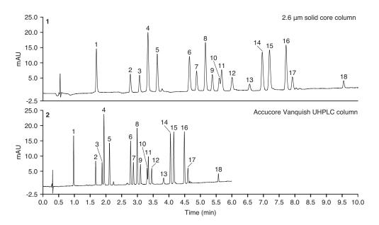
Figure 6: Chromatographic separation of 18 herbicides on a  $2.6~\mu m$  solid core column (top) and the Accucore Vanquish UHPLC column (bottom)
