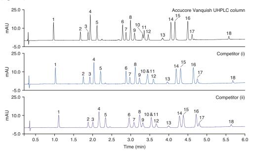
Figure 1: Chromatographic separation of eighteen herbicides on Accucore Vanquish UHPLC column (black), competitor (i) (blue) and competitor (ii) (purple) columns
