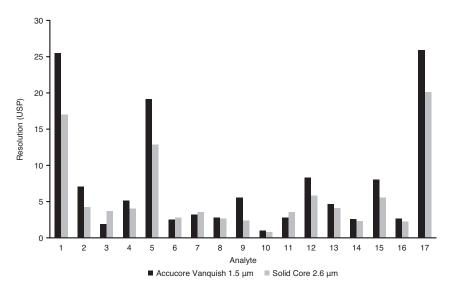
Figure 8: Comparison of resolution between the Accucore Vanquish UHPLC column and a  $2.6~\mu m$  solid core column
