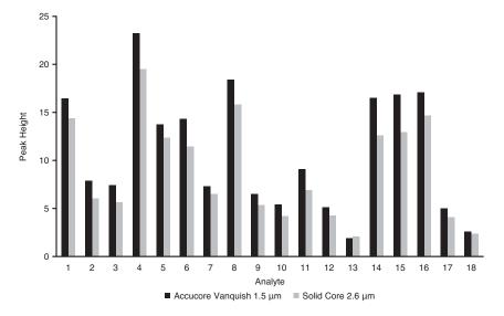
Figure 7: Comparison of peak height between the Accucore Vanquish UHPLC column and a 2.6  $\mu$ m solid core column
