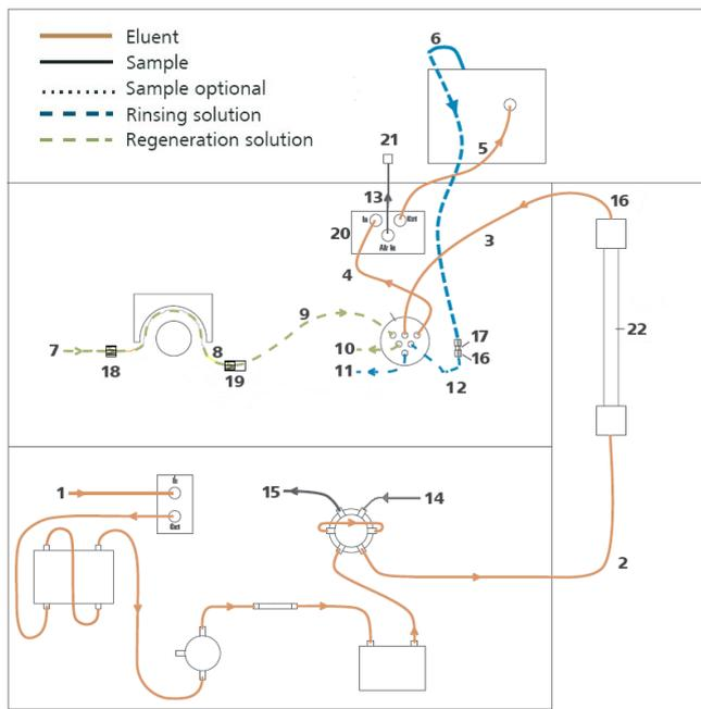
Make sure that all outlet capillaries are put into the waste collector (detector outlet, sample waste, suppressor waste, ...).
