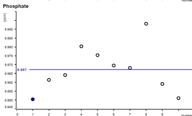
The precision of 10 injections of the 10 ppm standard was determined (Dilution factor 2). The results are shown in the following table and an exemplary trend chart is shown for Nitrite and Phosphate.
