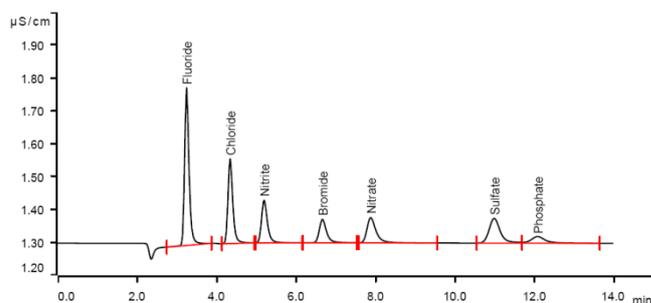
The calibration was performed with one standard containing standard anions of 20 ppm each. Within the concentration range of 0.2 – 10 ppm, a quadratic curve type was used for evaluation.
