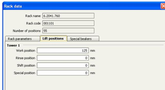
For using the Liquid Handling Station, it is necessary to define external positions for the needle. This is done in the configuration of the Sample Processor in the subtab “Tower”. Please define the external positions 1, 2 and 3 according to the picture below. Attention: The angles are only approximate values, for fine tuning, please use the
