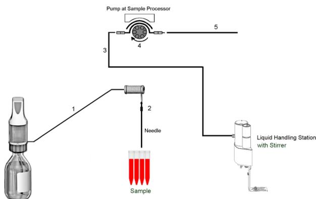
1. Transfer Tubing with holder 2 x M6 / 10 mL (6.1562.130) to be connected to Dosino port 1. The holder can be fixed as a chain element at the Tower. The other end is fixed to Adapter UNF 10/32 outer / M6 inner (6.2744.200) (see 2.)
