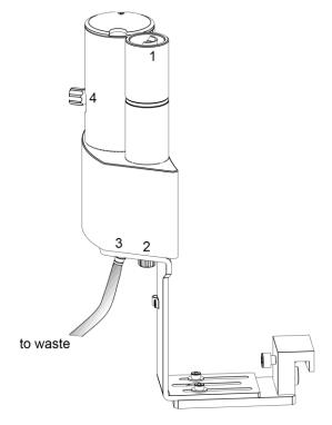
Number 4 of the picture above shows the attachment point of a capillary in case of a dilution feature and Number 1 indicates the rinsing entity.
