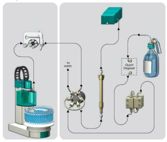
Prepare and degas an eluent suitable for the column you want to use (see column manual). For Metrosep Carb 2 - 150/4.0 a solution of 100.0 mmol/L sodium hydroxide and 10 mmol/L sodium acetate is adequate.
