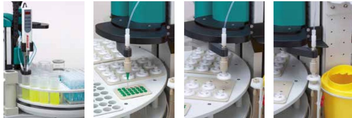
Automated sample preparation: In the first step, solvent is added and the sample is pulverized and homogenized. After that, sample is drawn up with a metal-free needle, filtered, and finally transferred directly to the IC system by way of a connection port.
