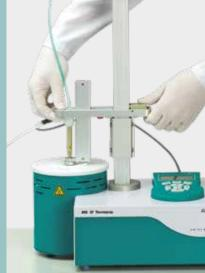
End of titration: After the titration the vial is removed from the oven
