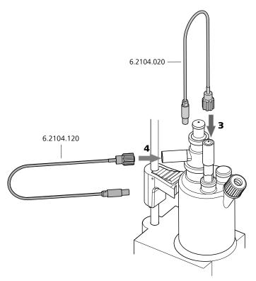
Figure 18 Screwing the electrode cable to the electrodes
