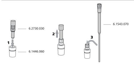
Insert the aspiration tip into the coulometer cell as follows:
