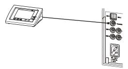
Figure 4 Connecting the Touch Control
