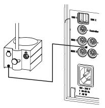
Figure 8 Connecting an MSB stirrer
