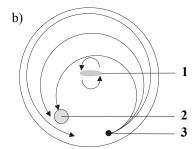
Figure 12 Schematic configuration of magnetic stirrer, indicator electrode and buret tip (Volumetry) /Generator electrode (Coulometry) during a titration. a) stirring direction clockwise, b) stirring direction counterclockwise.
