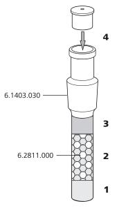
Figure 14 Filling the adsorber tube
