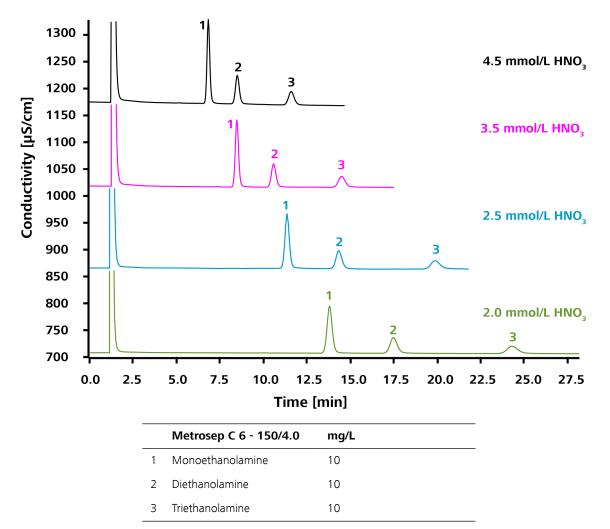
Increasing the nitric acid concentration shortens the retention time of the amines.
