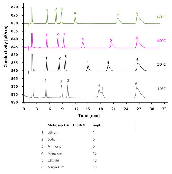
In the case of calcium, the complexation with the dipicolinic acid is weakened with higher temperature. This results in it eluting later. An increase in temperature results in slightly longer retention times for lithium and magnesium. The other cations such as sodium, ammonium and potassium elute earlier.
