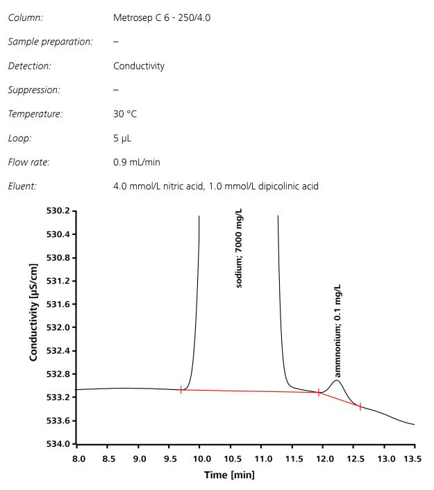
The very high sodium/ammonium ratio reached is 70,000:1 here.
