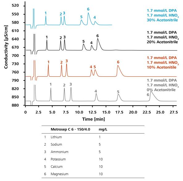
By adding acetonitrile to the eluent, the retention time of all cations is shortened, whereat the effect is more visible in divalent cations. When adding 10% acetonitrile, potassium and calcium co-elute. When adding 20% acetonitrile, calcium elutes before potassium.
