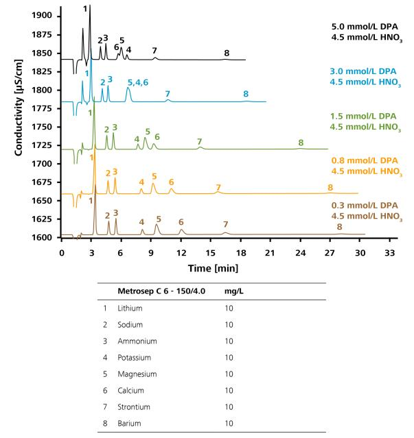
The addition of dipicolinic acid to the nitric acid influences the retention of calcium, magnesium, barium and strontium through complexation. Increasing the dipicolinic acid concentration accelerates these cations. The best separation is reached with 1.5 mmol/L dipicolinic acid. From 3.0 mmol/L dipicolinic acid, calcium, magnesium and potassium co-elute. At 5 mmol/L, calcium and magnesium elute before potassium.
