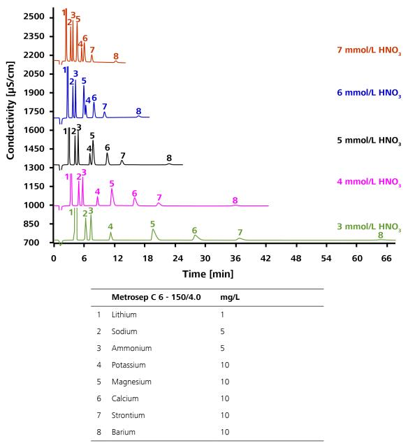
Increasing the nitric acid concentration accelerates all standard cations. The divalent cations are accelerated disproportionately. At 5 mmol/L, calcium co-elutes with potassium. From 6 mmol/L, magnesium elutes before potassium.
