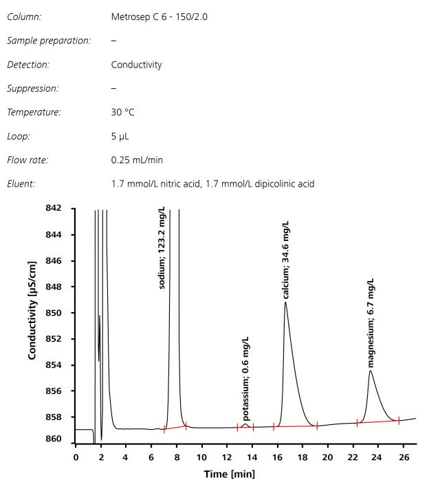
The sodium concentration is increased because this drinking water has been treated in an ion exchanger.
