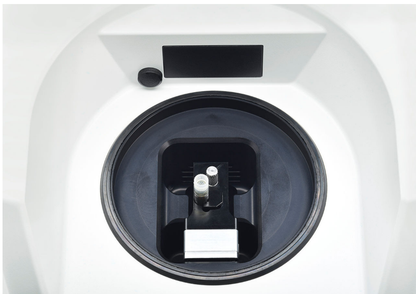
Figure 4 Place the disposable vial in the sample compartment.
