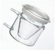
Heatable cell for titrations at elevated temperatures
