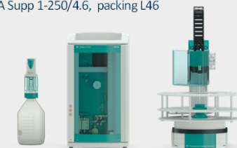
Fig 5. Ion Chromatography Instrument used for Fluoride Assay in OTC Products
