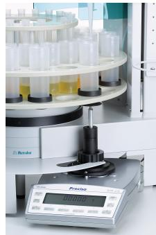
The patented technique of weighing the sample directly on the rack is unique. There is no simpler way to prepare a sample – just position it and press START. All other steps are carried out fully automatically by the system. This includes taring of the titration beaker as well as transferring the correct sample amount. This technique significantly improves the accuracy and reproducibility of the results.
