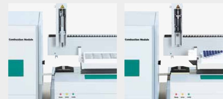
CIC automation. Solid or liquid samples – the MMS 5000 Autosampler can work with both.
