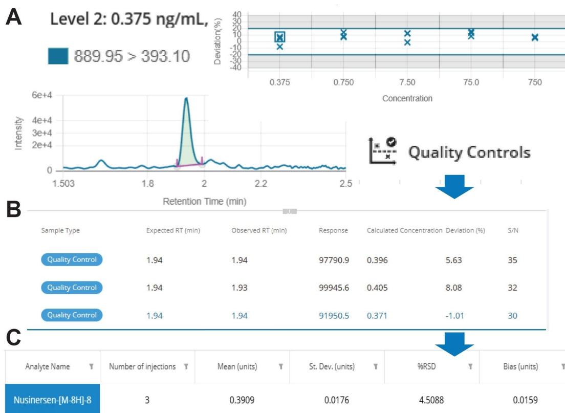
Figure 7. (A) LC/MRM chromatogram for nusinersen lowest QC level 0.375 ng/mL. (B) Quantitative information on the 0.375 ng/mL QC levels ( n=3 ). (C) QC statistics are calculated, and displayed for the lowest QC level.
