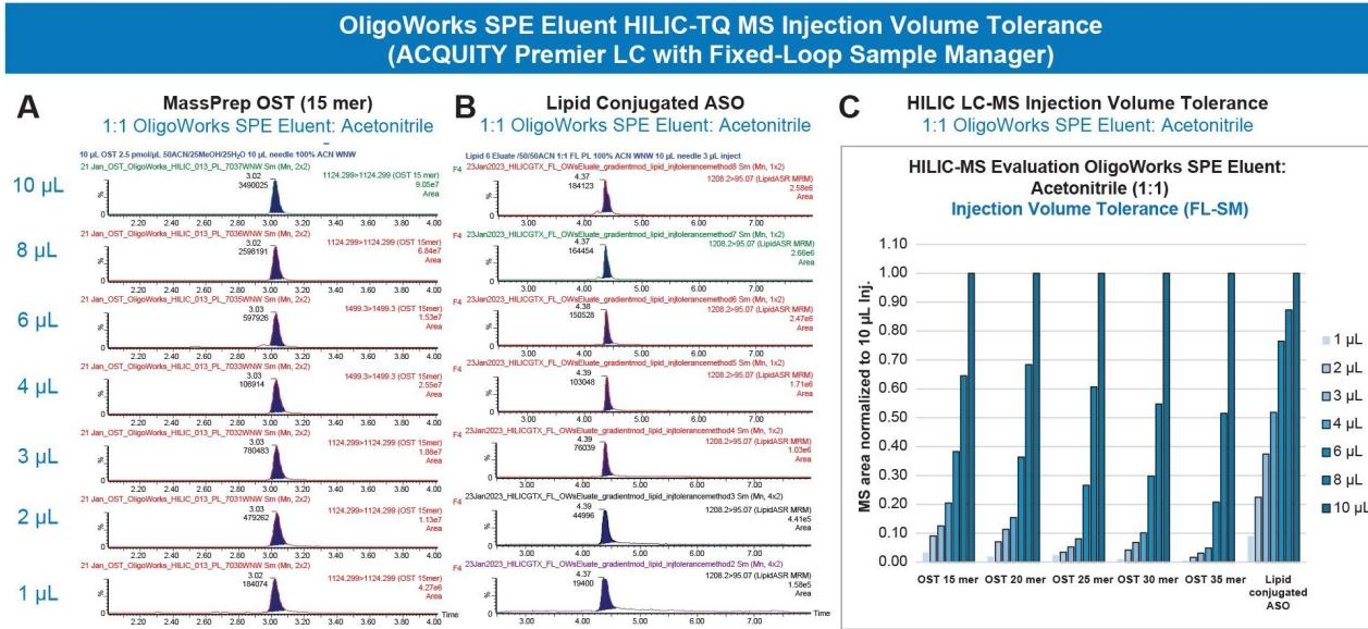
Analysis :ACQUITY Premier (Fixed-Loop Sample Manager 10  $\mu$ L Loop with partial loop pressure assist ,Injection mode)-TQ Absolute MS Systems
