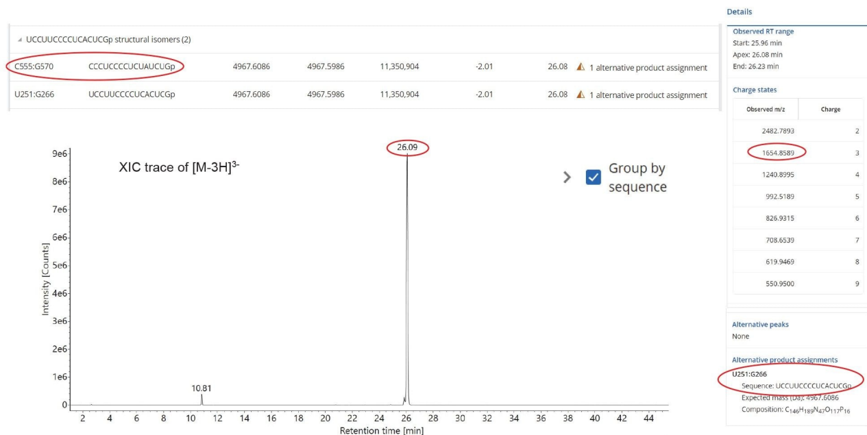
Figure 6. Extracted mass chromatogram of a triply charged precursor ( m/z=1654.86 ) that proves ambiguous as it could potentially be assigned to isomeric digestion products U251:G266 or C555:G570 resulting from RNase T1 cleavage of the GFP mRNA. The top inset shows the MAP Sequence assignment of these two structural isomers, while the right-side inset displays the charge states (2–9) detected by MAP Sequence for the ESI-MS spectrum of this oligonucleotide product.
