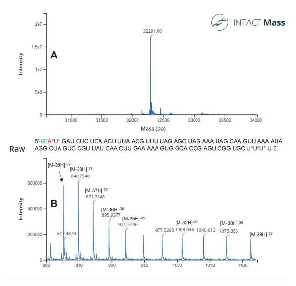
Figure 8. INTACT Mass spectra recorded for the most abundant 100-mer sgRNA oligonucleotide: (A) MaxEnt1 charge deconvolved spectrum; (B) raw ESI-MS spectrum.
