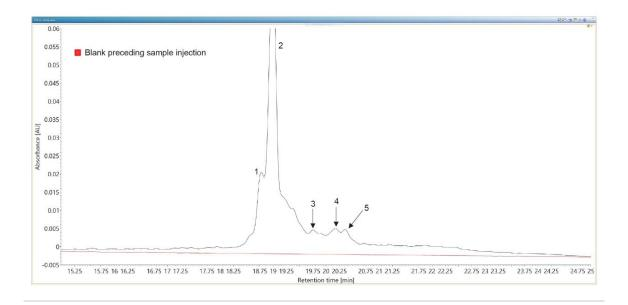
Figure 7. TUV chromatogram showing the separation of oligonucleotide impurities from a 100-mer sgRNA oligonucleotide. The sample was analyzed on a 2.1 x 100 Premier CSH Column using a 25-min gradient described in the Experimental section. The red trace corresponds to the blank preceding sample injection.
