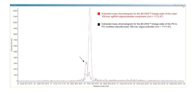
Figure 6. Overlaid extracted mass chromatograms recorded for an abundant charge state ([M-29H]  $^{-29}$ ) present in the major 100-mer sgRNA oligonucleotide (m/z = 1112.47, red trace), as well as in the most abundant impurity present in this sample, the PS to PO modified 100-mer (m/z = 1111.91, black trace). Both mass chromatograms were extracted using a tolerance of 0.1 Da.
