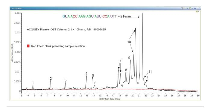
Figure 2. TUV chromatogram recorded at 260 nm, showing the separation of eleven oligonucleotide impurities from a 21-mer extensively modified chromatogram.
