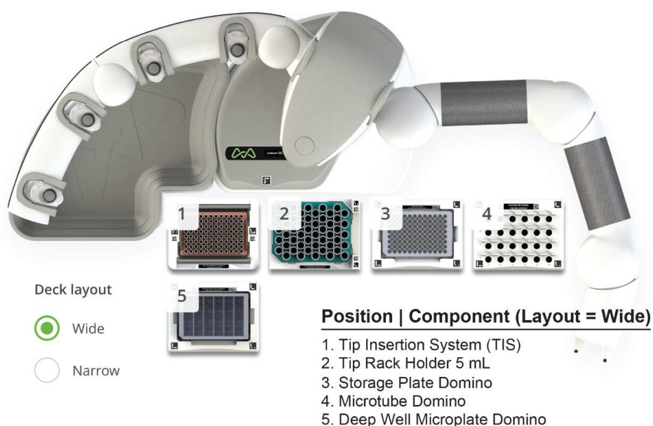
Figure 1. Andrew+ Pipetting Robot deck layout for serial sample dilution and calibration curve generation.
