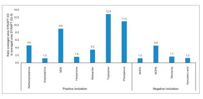
Figure 3. Response ratio between SYNAPT XS and SYNAPT G2-Si for 11 labile compounds (negative and positive ionization modes).
