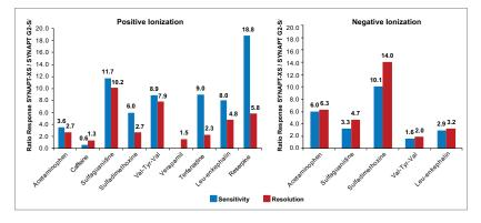
Figure 2. Response ratio between SYNAPT XS and SYNAPT G2-Si for the 9 compounds spiked into urine for positive and negative ionization. Sensitivity and resolution modes were utilized for both polarities.
