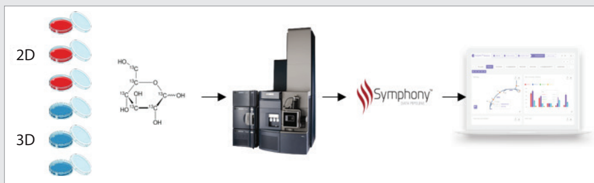
Figure 1. Graphical representation of the experimental design for the isotope labeling metabolic relative flux data analysis of 2D and 3D lung cells lines treated with 13 C-glucose using Symphony and Polly informatics.
