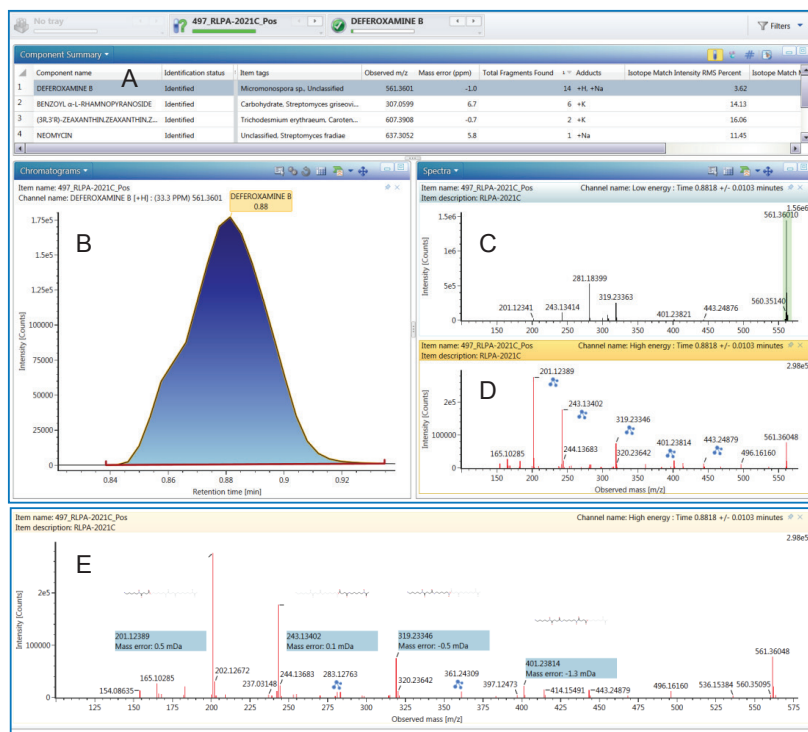
Figure 4. Compound identification result from the UNIFI microbial database. (A) The component summary interface; (B) Selected ion chromatogram of single component corresponding to panel A (C) The respective low energy precursor exact mass spectrum and (D) The corresponding high energy fragment ion spectra of Deferoxamine B with 14 matched fragment ion spectra. The blue "❄️" mark indicates the experimental fragment ion that matches to the expected in-silico fragment ions generated from the mol structure using MassFragment. (E) Zoom-in high energy display of likely structural fragmentation matches for Deferoxamine B.
