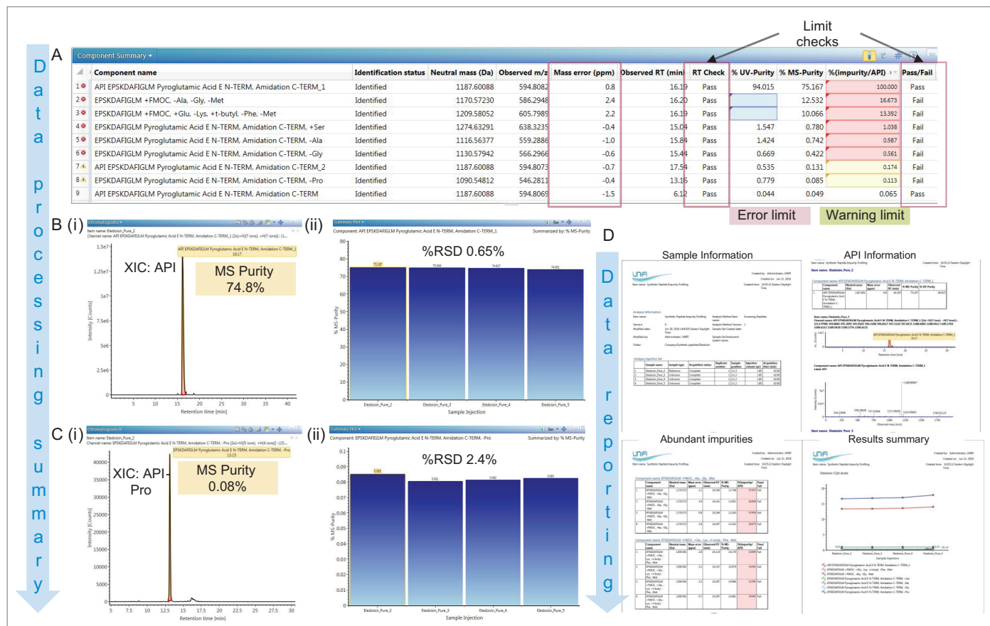
Figure 5. The figure shows the impurity profiling method in the screening workflow followed by the final report generated for the analysis. A) The panel shows the screening workflows' component summary displaying the purity level of API and each pre-selected impurity using both MS and UV detection. Using the features in UNIFI workflow method a pass/fail criteria display has been created to improve data readability. B) This figure displays the XIC (i) and the summary plot (ii) for Eledoisin API. C) The plot presents the XIC (i) and the summary plot (ii) for the impurity, API-Proline. The %RSD for both peptides are <3%. D) The reporting feature in UNIFI generates a consolidated report for the analysis. The reporting template can be user defined.
