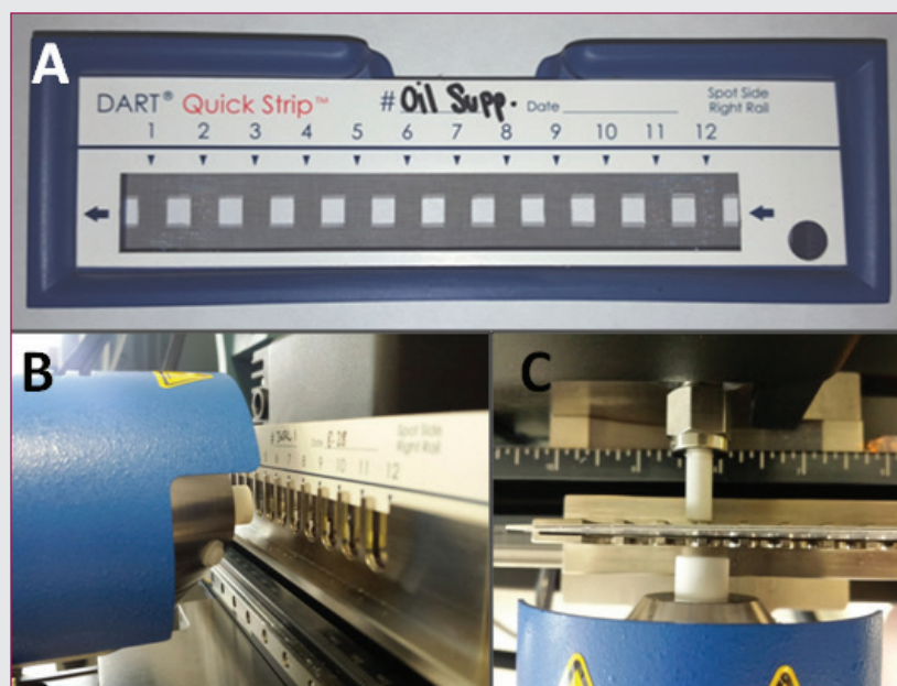
Figure 1. Images depicting A: the 12 spot QuickStrip card used for sampling; B: the QuickStrip card automatically being moved into the heated helium ionization beam; and C: the ceramic tube pulling ions into the QDa source (top down look at the DART source). The sample is applied to the QuickStrip card on the mesh screen in between each white open square.
