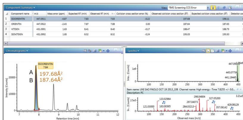
Figure 10. UNIFI Component Summary for Passiflora caerulea , illustrating coeluting isoorientin and orientin selected in the extracted mass chromatogram, with the corresponding precursor and ion mobility product ion spectra obtained. Mass measurement error <5 ppm, CCS errors <0.5% are presented. The extracted mass chromatogram shows the presence of a series of isobaric components between 7.0 and 11.0 minutes.
