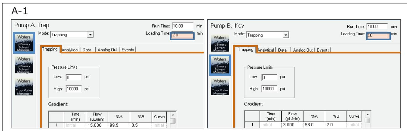
Figure A-1. LC pump mobile phase conditions when trap valve is set at trap position. The method shows that the trap pump is delivering 99.5% A/0.5% B isocratic to the trap column. The iKey pump is delivering 98% A/2% B isocratic, the initial gradient condition, to the iKey Separation Device. This is maintained for 2 minutes as shown in the “loading time” window.
