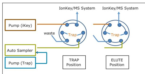
Figure 8. Instrument configuration dual pump trap-and-elute.
