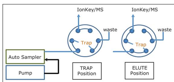
Figure 6. Instrument configuration using single pump trapping.
