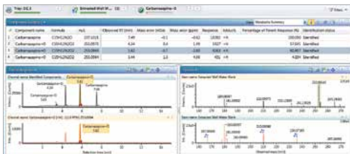
Figure 4. Full user interface (UI) information within UNIFI showing identification details of a proposed carbamazepine metabolite. Component Summary shows identification details while the chromatogram shows extracted ion chromatograms of all identified components with the component highlighted in the component summary. The spectra section shows precursor and fragmentation spectra for the highlighted component.
