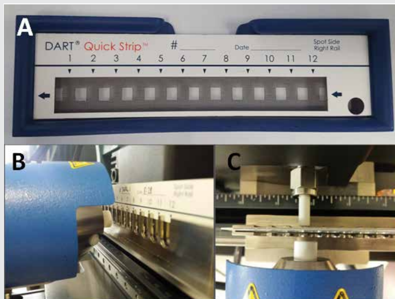
Figure 1. A. 12 spot QuickStrip card used for sampling; B. QuickStrip card automatically being moved into the heated helium ionization beam; and C. Ceramic tube pulling ions into the ACQUITY QDa source (top down look at the DART source).
