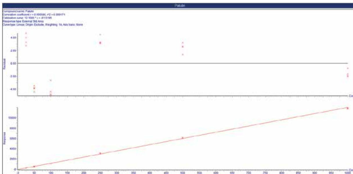
Figure 3. Calibration curve for patulin in extracted apple juice, equivalent to 5 to 200 \mu\text{g/L} .
