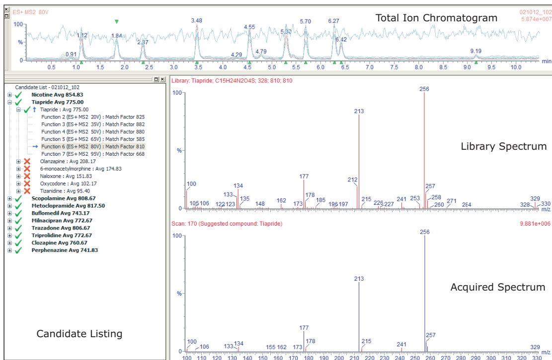
Figure 3. ChromaLynx browser displaying results of the full scan screening analysis of the SSM. Again, all ten components were detected, each one with a high average (Avg) match factor, indicating excellent agreement with the existing spectral library.
