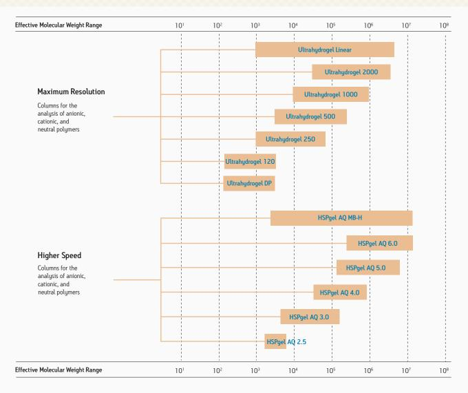
This chart compares the molecular weight ranges for the specified columns. By connecting two or more columns in series, the effective molecular weight range can be extended to provide coverage for more complex sample analysis.
