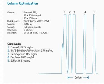
For optimum capacity and resolution, a 150 mm column is used in series with the 300 mm column. The use of both the 150 mm column and the 300 mm column provides maximum loading capacity while the 300 mm column provides maximum throughput and reduction in solvent consumption when used alone.
