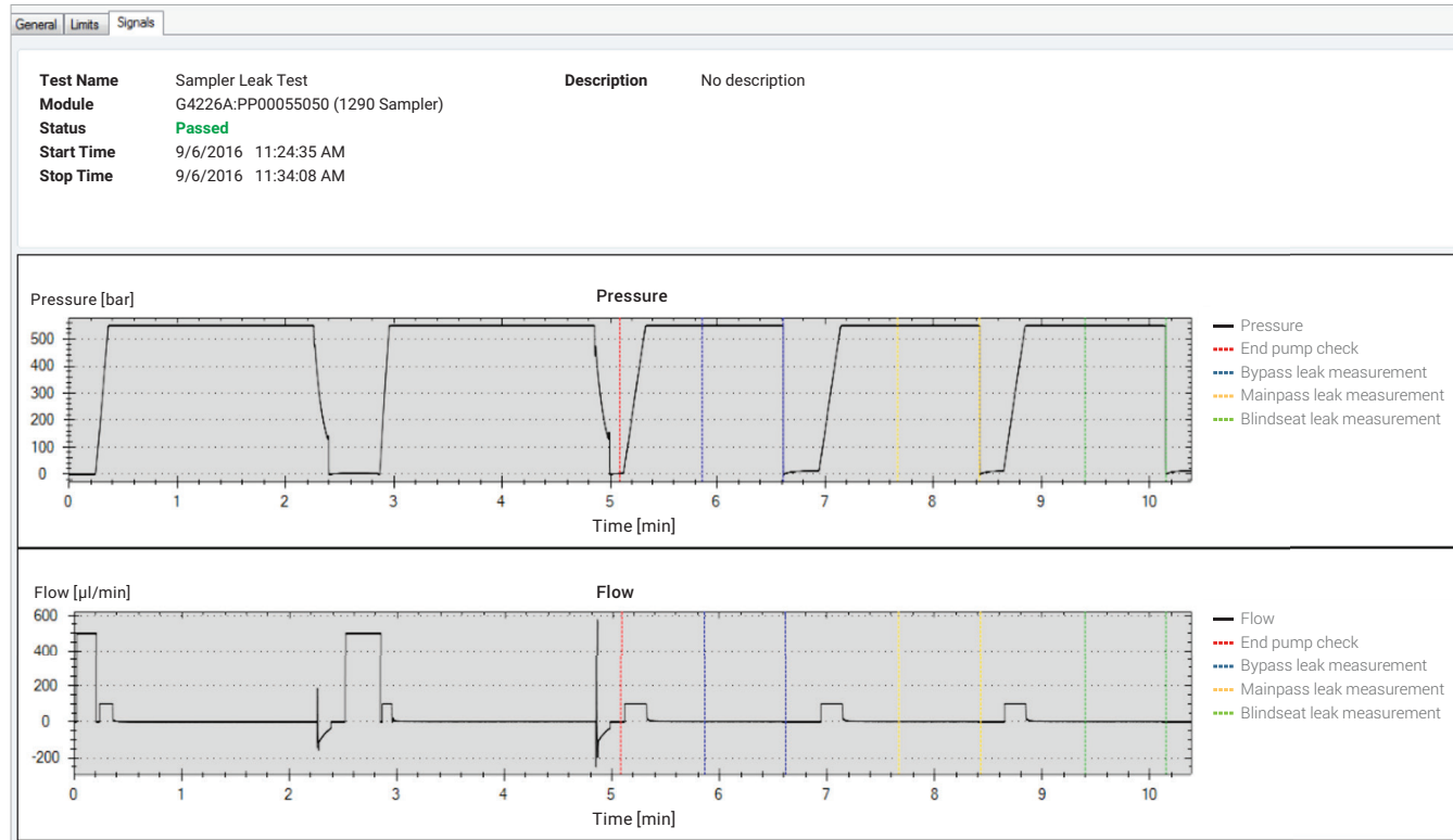
Figure 11. The Sampler Leak Test in Agilent Lab Advisor tests the specific leak rates of the rotor seal, metering device, needle seat, and system. The test requires that a blank nut gets installed at port 6 (outlet) of the injection valve. First, a pump head leak test is carried out on the selected channel, then a pressure test is carried out in the bypass position, then a pressure test is carried out in the mainpass position, and finally a pressure test is carried out in the mainpass position with the needle at the blocked seat position. At the end of the test, the results are evaluated automatically.
