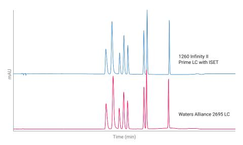
**Figure 3.** Overlay of a chromatogram acquired with the 1260 Infinity II Prime LC with ISET enabled and a chromatogram acquired with the Waters Alliance 2695 LC for the analysis of metoclopramide and impurities.
