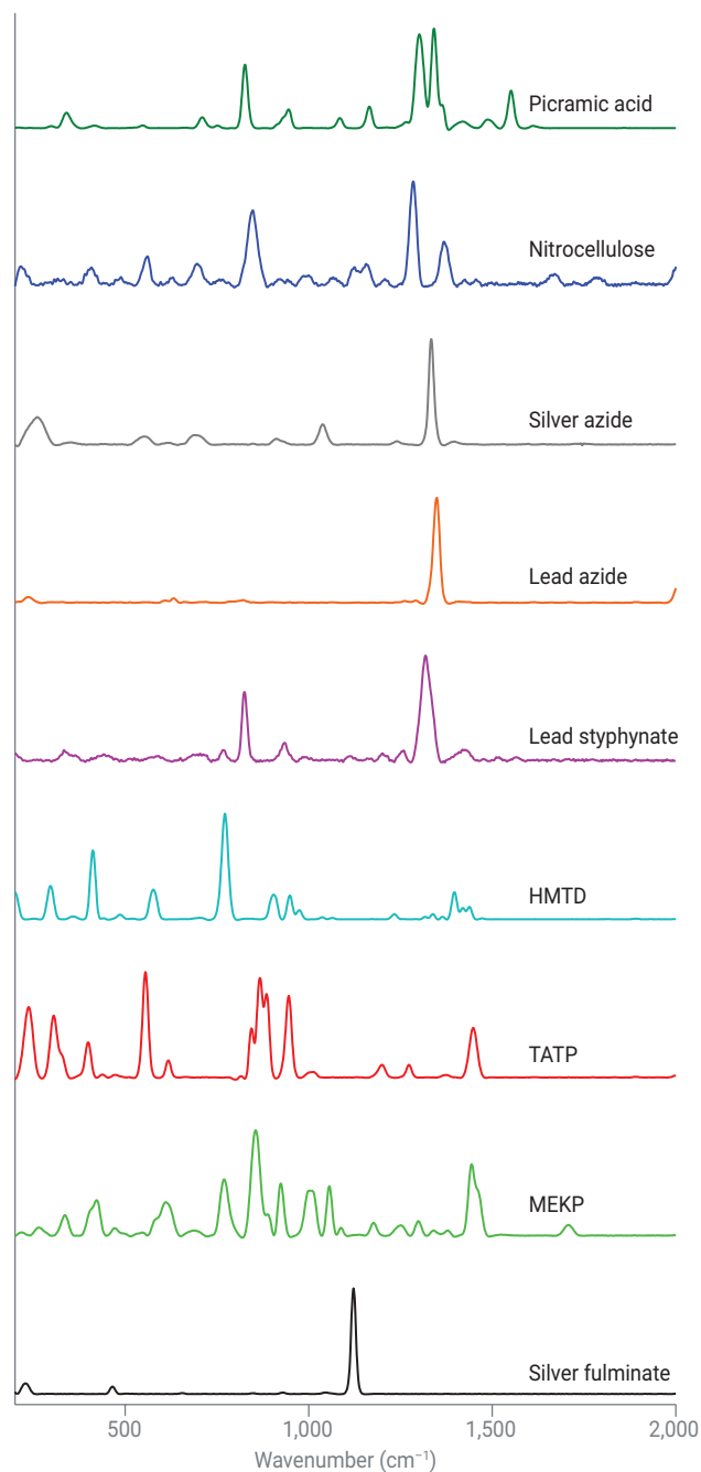
Figure 4. Example Raman spectra of nine primary and sensitive explosive materials, obtained during the Agilent Resolve system range testing. Measurements use point-and-shoot and vial modes.
