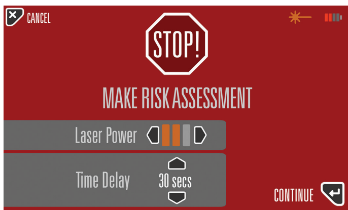
Figure 2. Risk assessment screen for setting a time delay or reducing laser power.
