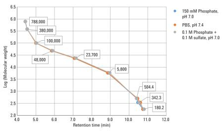
Figure 9. Effect of mobile phase composition on column calibration with polysaccharide standards.
