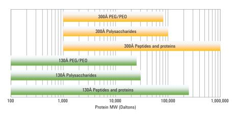
Figure 1. Resolving ranges for Agilent AdvanceBio SEC columns.
