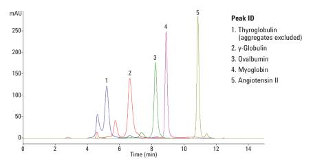
Figure 3A. Individual peptide and proteins contained in Agilent AdvanceBio SEC 300Å Protein Standard (p/n 5190–9417) on an Agilent AdvanceBio SEC 300Å column.
