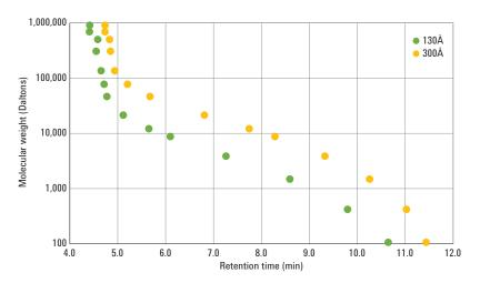
Figure 6. PEG/PEO Calibration on Agilent AdvanceBio SEC columns.
