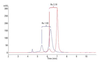
Figure 10B. γ-Globulin and BSA on an Agilent AdvanceBio SEC 300Å column using PBS, pH 7.4.
