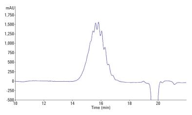
Figure 5C. Polysaccharide 5.8K run on Agilent AdvanceBio SEC columns  $300\text{\AA} + 130\text{\AA}$  in series.
