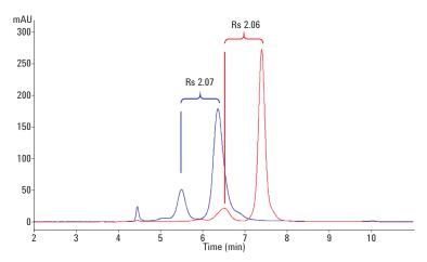
Figure 10A. γ-Globulin and BSA on an Agilent AdvanceBio SEC 300Å column using 150 mM sodium phosphate, pH 7.0.
