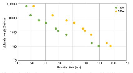
Figure 2. Peptide and protein calibration on Agilent AdvanceBio SEC columns.
