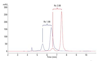
Figure 10C. γ-Globulin and BSA on an Agilent AdvanceBio SEC 300Å column using 100 mM sodium phosphate + 100 mM sodium sulfate, pH 7.0.
